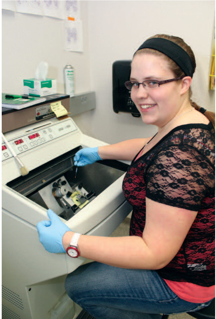
NMU student Rozemary Howard working on a cryostat machine that allows her to make very thin sections (12 micrometers) of a mouse brain, which she then places on slides and freezes at -80C to analyze messenger RNA, which may lead to advances in understanding neuromuscular diseases.
