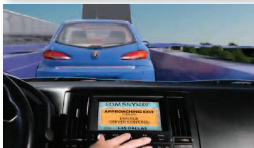
Vehicles would enter the Skyway from existing roads, and with a special component connect to the rail system, which magnetically and automatically transports the car at high speeds until the programmed exit is reached and the driver re-engages control.
