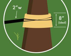
Using tree protection underneath the sling prevents damaging the bark.Tree protection should be around 8 Inches wide to account for up and down movement when the slackline is in use.
